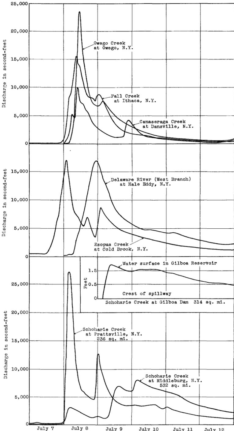
Figure 21.—Hydrographs of discharge at points in the Lake Ontario, Delaware River, Esopus Creek, and Schoharie Creek Basins, N. Y.
