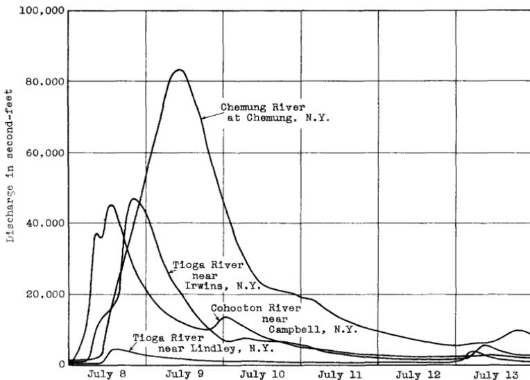
Figure 20.-Hydrographs of discharge at points in the Susquehanna River and Chenung River Basins, N. Y.
