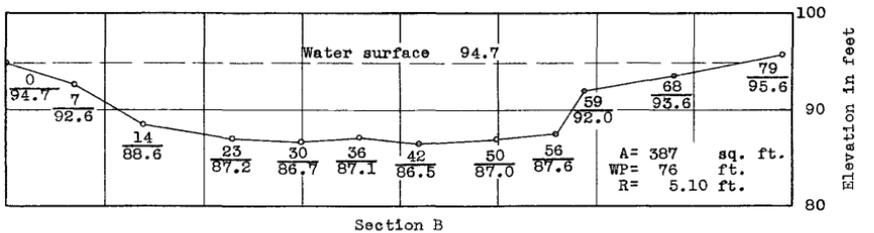
Figure 22.-Map, profile, and sections of slope-area reach on Glen Creek near Townsend, N. Y.
